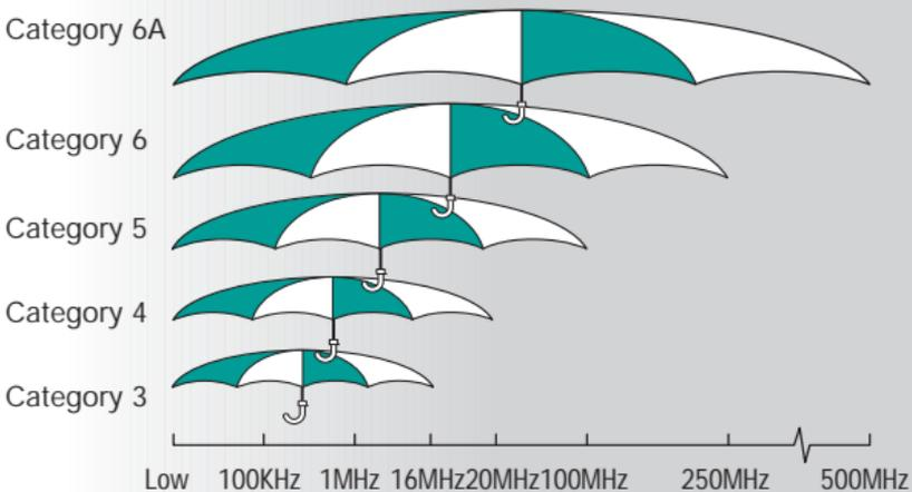
For new installations, **Category 6A** or Class E<sub>A</sub> cabling guarantees **10GBASE-T** support to 100 m over **UTP**. Since the international Class E<sub>A</sub> specification is more stringent, cabling for new installations intended to support **10GBASE-T** should be specified to meet the Class E<sub>A</sub> requirements.
