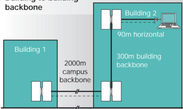
It is important to note that these maximums apply to all media. They do not take into account the performance differences between cable types and transmission protocols used by the network. In practice, maximum cable lengths will depend on the **application**, the type of network used (e.g. 1000BASE-T) and the cable's quality. Good cable suppliers and installers will advise on a **cabling** system's capabilities in a particular network.
