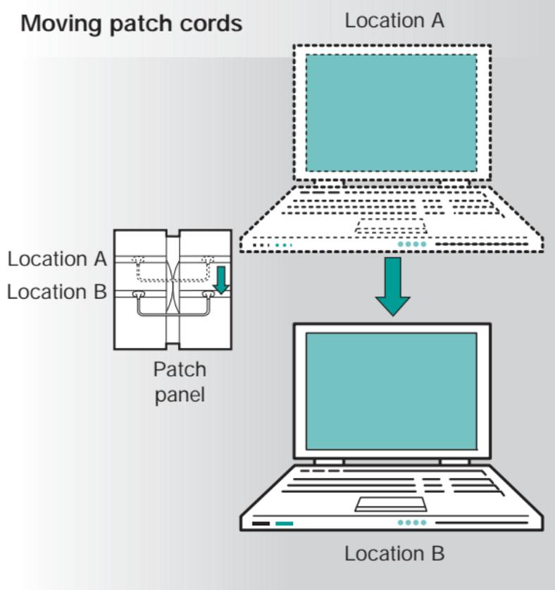
Between the outlets at the periphery of a network and the switches at its center there will invariably be patch panels. These allow cable runs to be connected and disconnected very quickly, simply by moving patch cords.
