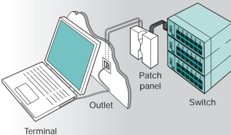
CENELEC EN50174 and TIA/EIA 569 cover many aspects of **outlet** location for mounting in walls, floors and furniture. In addition to standards criteria, accessibility must be considered.
