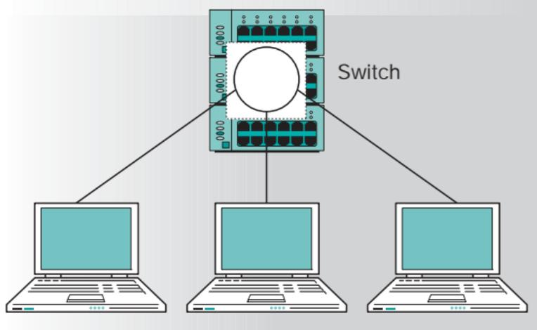
An example of this can be seen in the diagram above. The system shown has the appearance of a star, but its logical **topology** remains a true ring, with the loop completed within the central switch. Networks based on star, bus and ring type logical topologies all have their advocates, and the final choice largely depends on the **application**. The **star physical topology**, however, is now almost universally accepted within commerce and industry.
